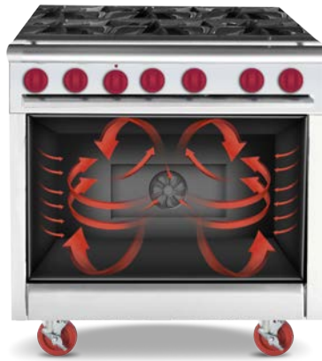
CONVECTION OVEN - C Convection High Volatility Air
